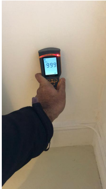
High moisture meter readings were noted on the wall in the front bedroom
